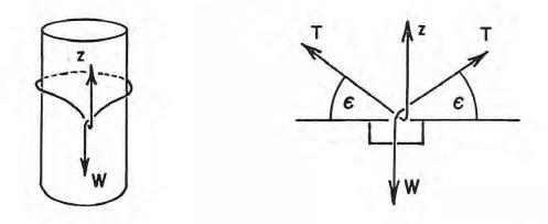
In equilibrium at the junction, the horizontal components of the tensions are equal and opposite. The vertical components will balance, too, when
