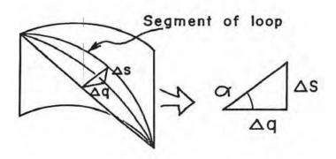
We get a little right triangle as indicated, when we draw a new straight line connecting the corners of the bent rectangle. This new line lies in the true plane of curvature of the short piece of loop. And more important, the angle  $\alpha$  is just the angle between this plane of curvature and the local perpendicular to the cylindrical surface. We see that
