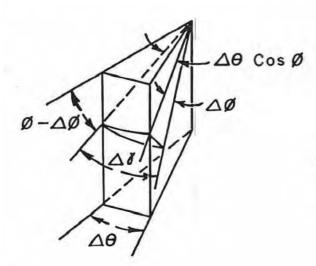
$(\Delta \gamma)^2 = (\Delta \theta)^2 \cos^2 \phi + (\Delta \phi)^2$  $\Delta \gamma = \sqrt{(\Delta \theta)^2 \cos^2 \phi + (\Delta \phi)^2}$ or  $\Delta \gamma = \sqrt{\cos^2 \phi + (\frac{-\mathrm{d}\phi}{-\mathrm{d}\theta})^2} \Delta \theta$
