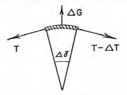
We have seen how  $\Delta \gamma$  is related to  $\Delta \theta$  and  $\Delta \phi$ . For the small angle  $\Delta \gamma$ , we may calculate  $\Delta G$  easily from the force diagram. Since  $\Delta T$  is very small,
