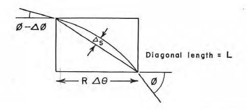
The diagonal of the rectangle is drawn. The separation  $\Delta s$  between the loop and the diagonal may be found by letting the arc be part of a circle, and noting that  $\Delta \phi$  is small.
