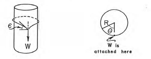
We have to use some kind of coordinate system. Looking down on the cylinder, the angle  $\theta$  designates a direction out from the center. We may let  $\theta$  be zero at the point where the weight W is supported, and it will then equal  $\pi$  radians (or 180°) around back at the most distant point. By stating a value for  $\theta$ , we refer to a particular point on the loop.
