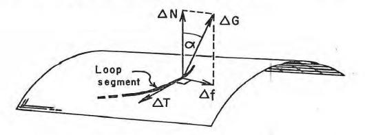
Both  $\Delta f$  and  $\Delta T$  are in the plane tangent to the cylinder. But  $\Delta N$  is perpendicular to this plane. The resultant force *in* the plane is the vector sum of  $\Delta f$  and  $\Delta T$ , and has the magnitude:
